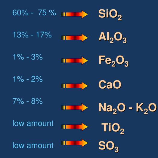
Its hardness is about to 5.5 to 6 according to the MOHS HARDNESS SCALE and does not contain crystallised water
