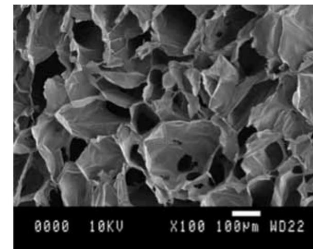
FIGURE 1. A micrograph of a collagen scaffold with isotropic pore structure at 100x magnification.
