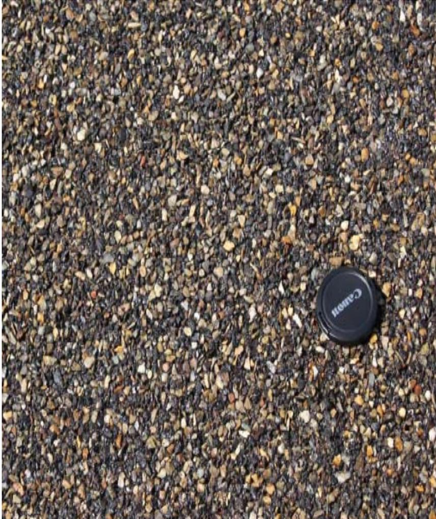
The material comprises of a stone rich mix that uses an aggregate selected for its visual appearance in addition to its engineering properties. Once the material has been laid, using conventional equipment and techniques, the bitumen is removed from the finished surface of the asphalt by shotblasting thereby exposing the colourful aggregate within the asphalt.
