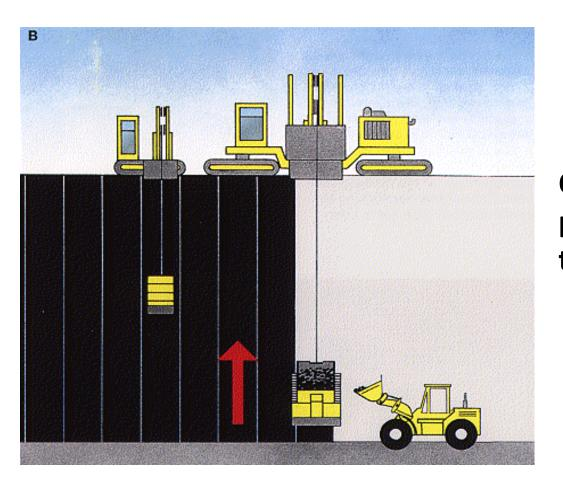
On smaller slopes the paver can be fed from the base.
