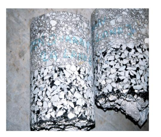
Cores showing the difference in grading between the dense asphaltic concrete (DAC) layer and the open graded asphaltic binder (ABL) layer. The right hand core shows particles of the drainage material still attached.
