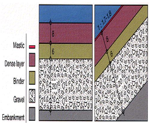
An asphaltic lining system would typically consist of;
