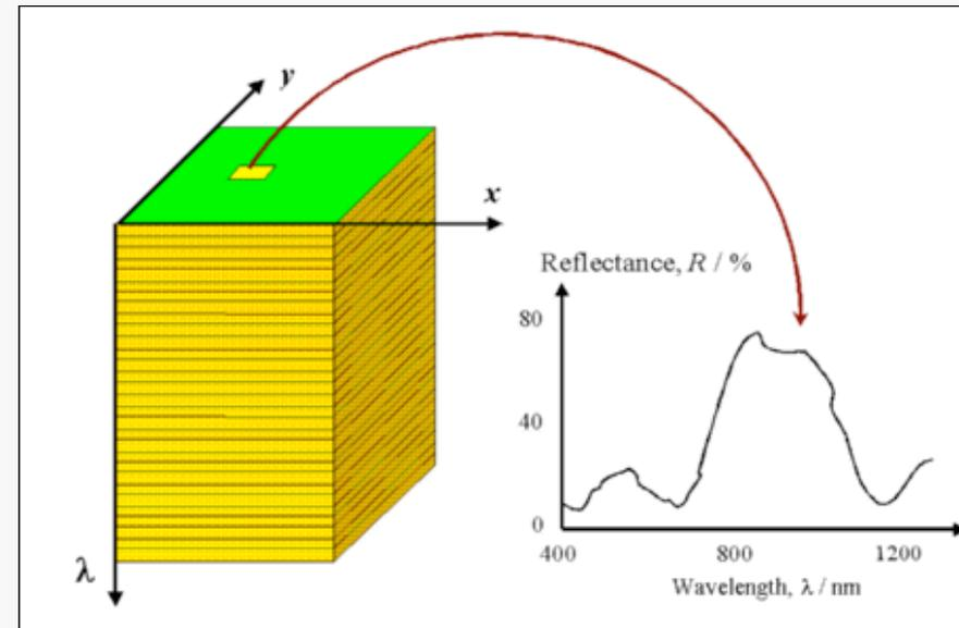
HSI emerging platform technology that integrates conventional computer vision and spectroscopy. It combines the advantages of both technologies by providing spatial, spectral, and multi-constituent information, while also being sensitive to minor constituents.
