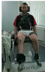
Figure 1: Subject seated in Biodex dynamometer. The leg rests on a mechanical arm and is secured with a Velcro cuff.
