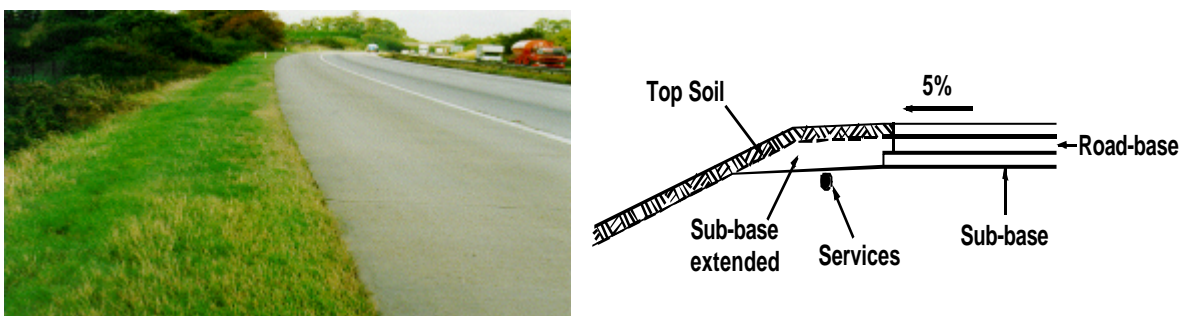
Figure 4: A typical scene of over-the-edge drainage and a layout of its construction
