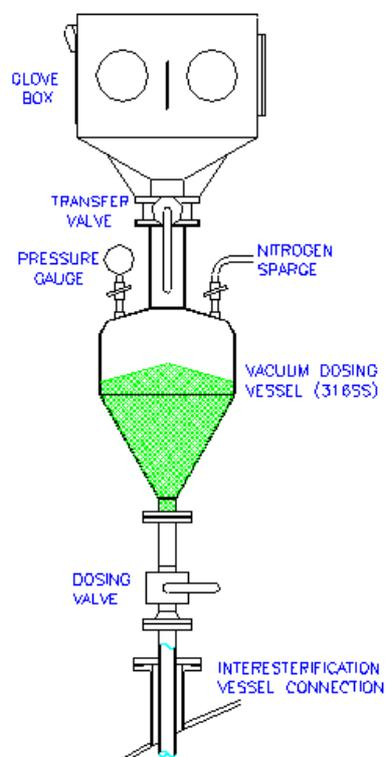
**Figure 2.** Catalyst dosing system design
